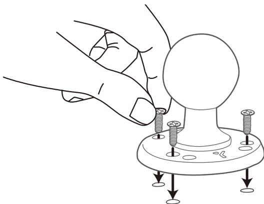
Align existing AMPs holes and attach with screws (not included)
