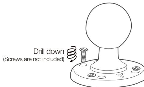
Using appropriate screws for the surface (not included), drill down the base
