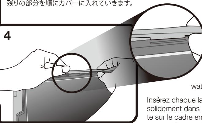
Insert each silicone tab tightly into its corresponding slot in the hard frame to ensure the case is water-resistant.
